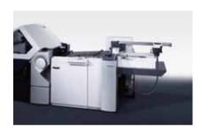
Flat-pile feeders are designed to accommodate frequent folding job changes and short to medium runs. Lateral blowers and the Tremat sheet separator ensure perfect sheet separation and aeration of the feed pile. A polyurethane-coated suction wheel then feeds the sheets one by one onto the register table. Formats are quick and easy to change from job to job. Other benefits include a small footprint and low investment costs.
