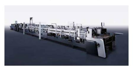
The Diana® X 80 and Diana X 115 folding carton gluing machines can be used flexibly for the production of both standard and high-quality packaging. With production speeds of up to 650 meters (2,130 feet) per minute, a high level of automation, and an open and easily accessible modular design, they deliver maximum productivity, precise folding carton processing, and optimum flexibility. This innovative technology makes it possible
