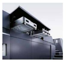
With the DryStar® UV, the benefits of the DryStar system can also be used in UV printing. Its perfect integration into the press, the very small distance between UV dryer and sheet, and the use of an innovative reflector coating have made it possible to increase the dryer output significantly. As a result, top production speeds are possible in UV printing, too.
