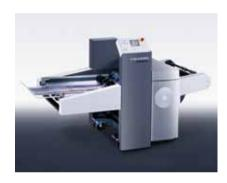
The SPH stream delivery has an integrated pressing device. The individually adjustable upper and lower conveyors gently remove the signatures from the folding machine.
