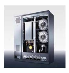
AirStar® and ScrollStar® are perfectly coordinated with Speedmaster® presses. AirStar combines virtually all individual blowers providing vacuum and blast air in a single, central air supply cabinet, while ScrollStar ensures that the supply of compressed air to the press is completely free of oil and condensation.
