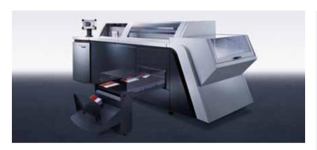
The Eurobind® 600/600 PUR sets new standards in adhesive binding for runs of up to 2,500 copies. All key functions are controlled on a central touchscreen. Based on the entries made on this touchscreen, the Eurobind 600/600 PUR automatically adjusts the clamp opening width and glue application to the block thickness. The unique spine preparation station with its combination tool optimally prepares blocks for glue application. Precise, uniform gluing ensures
