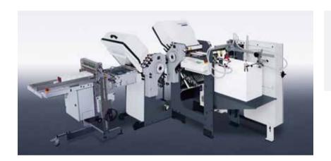
The Stahlfolder® Ti 36 is the specialist machine for very small folds. It satisfies the most demanding requirements for very short folding lengths and makes it possible to move into lucrative markets such as pharmaceutical packaging inserts. The available options allow a single operator to execute a wide variety of different folds.
