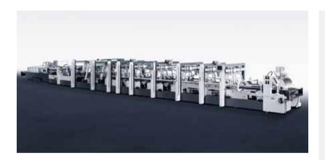
The Diana® X 135 is an advanced folding carton gluing machine with a modular design that achieves top levels of automation. A turning module enables blanks to be rotated clockwise or counterclockwise by up to 180 degrees (depending on the format), in many cases eliminating the need for a second pass through the machine. Other features that ensure exceptionally user-friendly operation include a touchscreen with graphic
