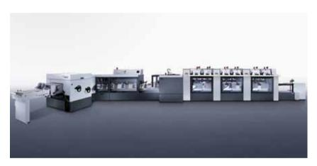
The Stitchmaster® ST 100 ensures cost-efficient finishing of short and medium runs with constantly changing formats. Operating at up to 9,000 cycles per hour, the machine produces professional results in formats up to A4+ and enables print shops and bookbinders to cover the entire production chain.
