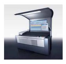
Its high degree of automation quickly makes Prinect® Axis Control® an indispensable helper at the press in any print shop. Simultaneous color control of all ink zones is based on values calculated spectrophotometrically. Especially in combination with the new digital ink zone drives in the Speedmaster® model series XL, CX and SX, the press inks up much faster and less waste is produced during makeready and production run
