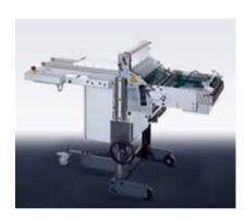
The mobile STA 40 delivery system was specially designed for easy handling and optimum delivery of small-format products with a final length of up to 2 centimeters (0.79 inches). A brake in the pile magazine prevents the signatures from "popping up", while a marking device staggers the pile laterally into clear, counted batches. The travel mechanism has gear racks for smooth adjustment to any height required.
