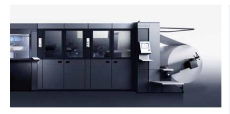
The cost benefits of web offset and the flexibility of sheetfed offset – the CutStar® sheeter offers you the best of both worlds. CutStar is installed right in front of the feeder. It allows you to process grammages of between 40 and 300 gsm. The printing stock is unwound from the reel, cut to the required format in CutStar, shingled, and fed into the feeder. The feed process is extremely reliable and stable. By using less expensive reel
