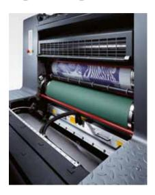
Prinect<sup>®</sup> Auto Register measures register while the press is operating, ensuring optimum register from the very first pull.
