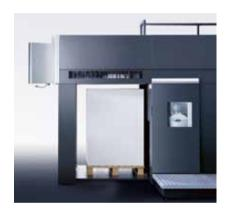
The CleanStar® powder extraction system from Heidelberg® was developed specifically for Speedmaster® presses. Its operation and performance have been geared precisely to the press's specific requirements. CleanStar minimizes powder emissions from the delivery. This results in 80 percent less dust around the press. CleanStar also reduces possible odor emissions resulting from the use of dispersion coatings.
