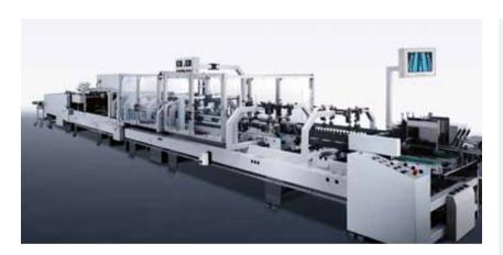
The Easygluer® 100 was designed as a universal machine for professional applications. Even the standard configuration can output up to 50,000 lockbottom cartons per hour at speeds as fast as 300 meters (just under 1,000 feet) per minute, in addition to producing straightline and double-wall cartons. The option of extending its capabilities to fourand six-corner collapsible cartons and adding special tools also makes it possible to tap
