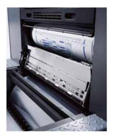
Prinect® Inpress Control automatically measures color and register on the fly. Integrated directly in the press, the measuring unit measures process colors, spot colors, and register in the print control strip. Any corrections required are forwarded directly to the Prinect Press Center® press control station for
