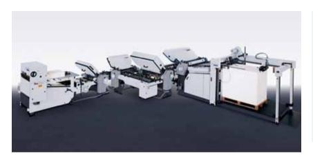
The folding machines in the Stahlfolder® TD range are ideal for processing large and special formats. When used in conjunction with the optional twin-lay attachment for simultaneous processing of two repeats – possibly with different contents – these folding machines boast outstanding productivity. The mobile folding units can be arranged either at right angles or in a line. These folding machines can be used with both pallet
