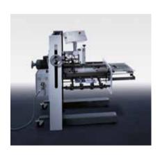
It is common for bookbinders to require an extra folding unit for a quick and easy additional cross-fold. The VF 66 four-directional folding unit is particularly well-suited to this task. It is mobile, which makes it flexible for use with other finishing equipment. The unit's greatest strength is its working width of up to 66 centimeters (25.98 inches), which enables it to be used as the last folding unit for map production or placed after a thread-sealing machine or saddlestitcher.
