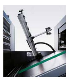
Clean sheet separation, optimum sheet travel, and exceptionally high production speeds are only possible if your printing stock is free of electrostatic charges. This is particularly important for low grammages, coated materials and, above all, plastic films. StaticStar® from Heidelberg® is the ideal solution. It cuts the electrostatic charges of sheets and stabilizes the production run. StaticStar Compact is designed for everyday substrates such as paper and cardboard.
