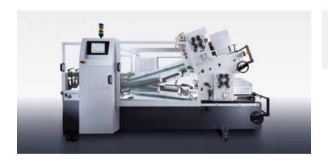
The Inlet-Spotter module enables reinforcing inlets to be glued into folding carton blanks, for example in the case of large soap powder boxes or two-part packaging used for transport and display purposes. The timed feeder of the Inlet-Spotter ensures greater reliability and flexibility in the production of two-part packaging. Operating at speeds of over 200 meters (650 feet) per minute, it sets the correct speed for the folding carton gluing
