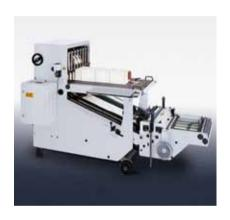
The key benefit of the SBP horizontal stack delivery is that its large capacity – made possible by arranging piles horizontally on the long pile board – makes it ideal for medium and long runs. It also enables cost-effective one-person operation of both the folding machine and delivery in tandem.
