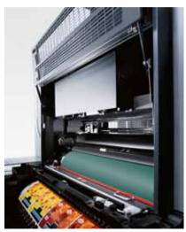
Premium quality calls for highly accurate control. Designed for the Speedmaster® model series XL 106, CX 102 and XL 75, the Prinect® Inspection Control inline sheet inspection system seamlessly controls and documents the entire print run at full production speed. Prinect Inspection Control
